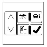
The Driver Information Center (DIC) has different displays which can be accessed by pressing the DIC buttons located on the instrument panel, to the left of the steering wheel.
